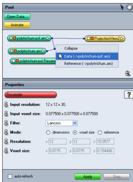
Figure 1.2: Resampling a PSF using the Resample module.
